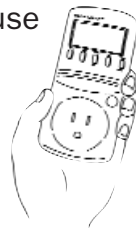
This device, a wattmeter, when placed between an appliance cord and wall outlet, will measure the energy the appliance uses.
